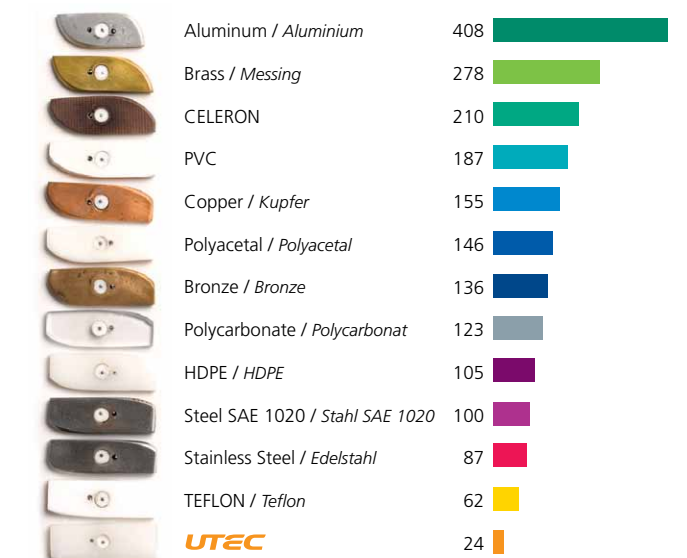
Figure 4 – Relative abrasion wear of UTEC grades and various materials, STEEL SAE 1020 = 100. The pictures show the tested parts. Measured by Braskem internal sand-slurry method.
