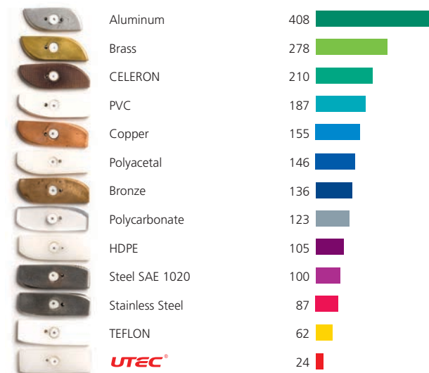
Figure 4 – Relative abrasion wear of UTEC grades and various materials, STEEL SAE 1020 = 100. The pictures show the tested parts. Measured by Braskem internal sand-slurry method.
