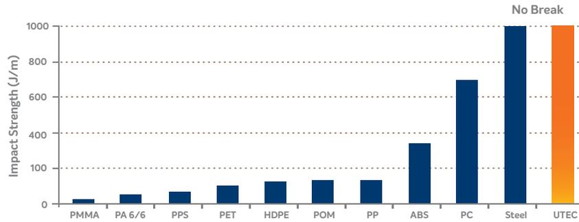
Figure 1 – Notched Izod Impact Strength (ASTM D 256): UTEK vs. other materials.
