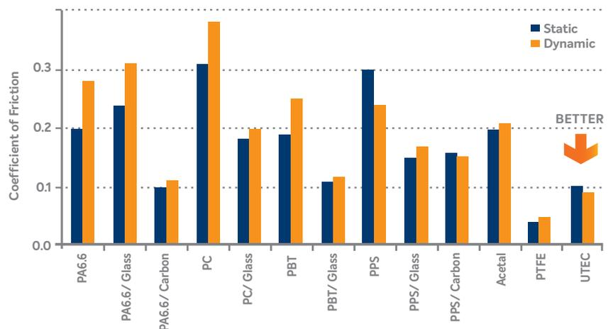
Figure 2 – Static and Dynamic Coefficient of Friction of UTEK and other materials.
