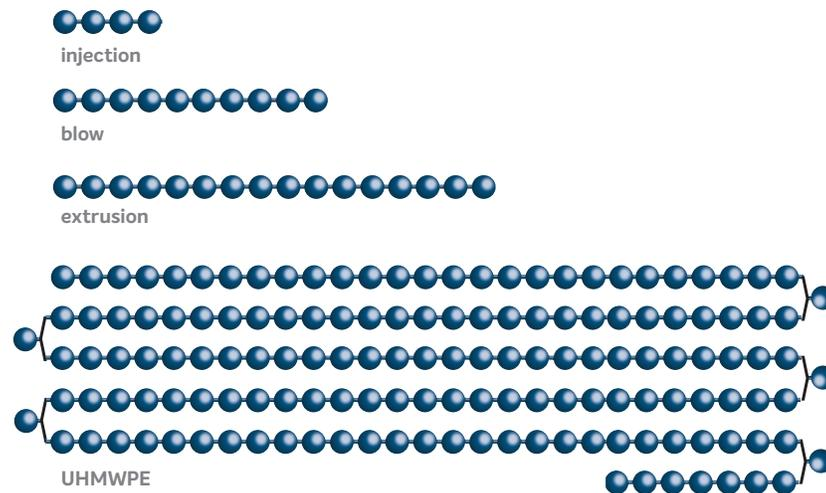
Figure 3 – Comparing polyethylenes for injection, blow and extrusion molding with UTEC® UHMWPE polymeric chain
