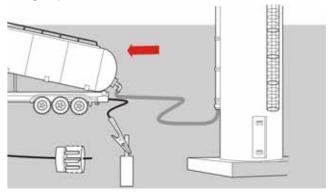
4. The truck bracket should be activated before tilting the trailer. Only after all connections are made and checked, start unloading and tilting the trailer.
