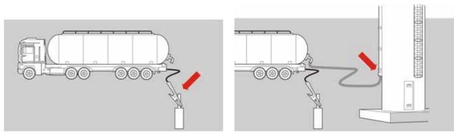
1. The truck should be grounded with the appropriate ground cable connection.
