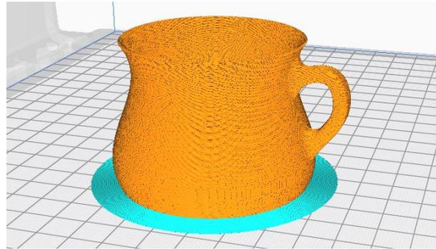
The brim width required will depend on the part geometry being printed. At least a 5-layer brim width is recommended to start, but this number should be increased for more complex or warpage-prone geometries.
