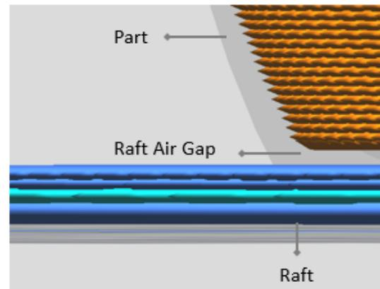
**Raft Air Gap:** The most important parameter is the raft air gap. The raft air gap is the spacing between the topmost layer of the raft and the bottom most layer of the part. The ideal set point for the raft air gap is 0.1mm (this value may vary slightly up or down based on your printer's make and model).
